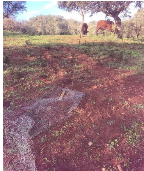
Figure 3. Erosion measuring device completely destroyed.
