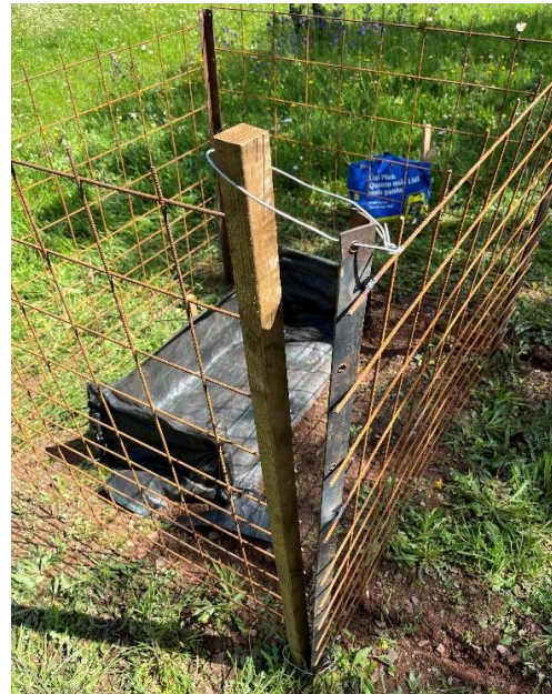
Figura 5. Erosion measuring protective grid and its opening for collecting material.
