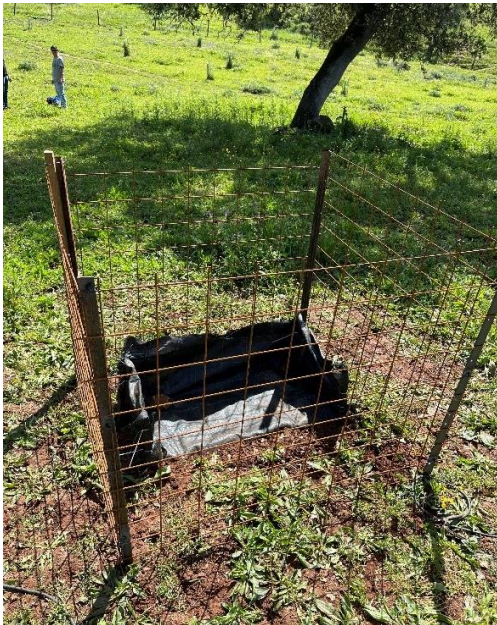
Figure 4. Erosion measuring device restored and isolated from animals.
