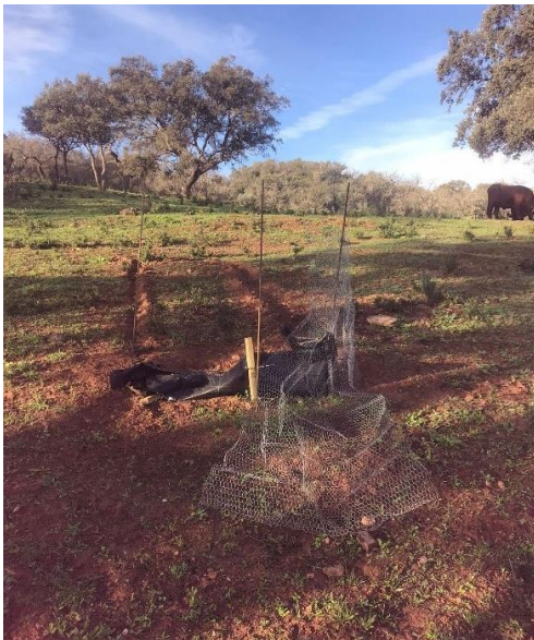
Figure 2. Erosion measuring device partially destroyed.
